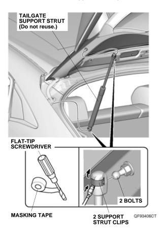
8. With the help of an assistant, install the new tailgate support strut to the two bolts.
