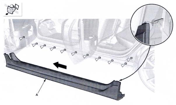
4. Remove the clips (B) from the body by turning them 45  $^{\circ}$ , then install them to the side sill panel.
