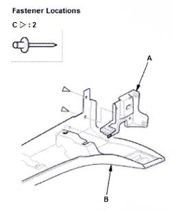
1. Install the side sill panel support (A) to the side sill panel (B) with the new rivets (C).
