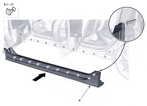
3. Install the screws (A) and the clips (B).
