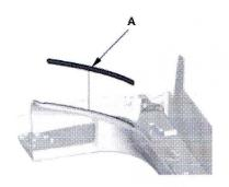
1. Install the side sill panel lip seal (A).
