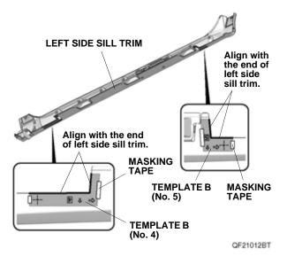
17. Using a pushpin, pierce the center of the mark on each template B.
