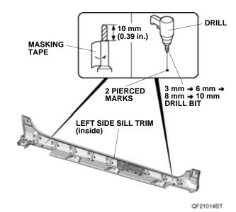
20. Using a file, remove any burrs from the holes.
