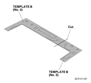
16. Line up template B No. 4 and No. 5 with the left side sill trim as shown and attach them to the left side sill trim using masking tape.
