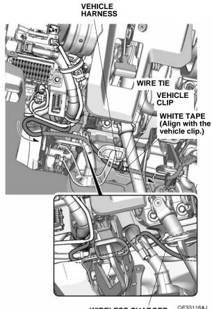
WIRELESS CHARGER QE33116AJ HARNESS 42. Secure the wireless charger harness to the vehicle harness with three wire ties.
