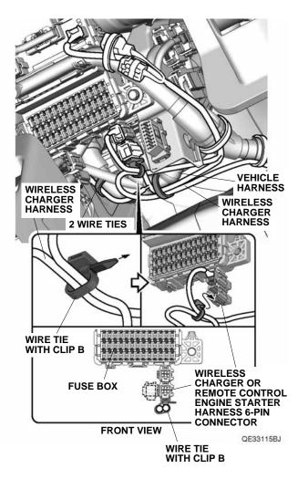
40. Secure the wireless charger harness to the vehicle harness with two wire ties. Go to step 45.
