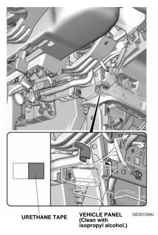
23. Attach the other piece of urethane tape to the vehicle panel.
