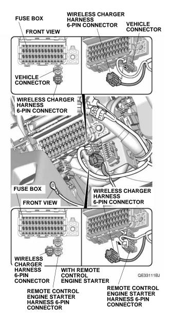
36. Remove the vehicle ground bolt and install the wireless charger harness ground terminal with vehicle ground bolt as shown. Do not put the ground terminal calking on top of one another.
