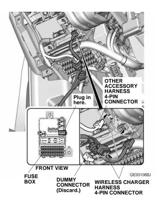
28. Plug the wireless charger harness 4-pin connector into the fuse box.
