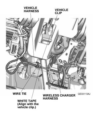
38. Secure the wireless charger harness to the vehicle harness with two wire ties.
