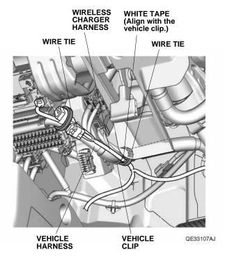
30. Secure the wireless charger harness to the vehicle harness with one wire tie.
