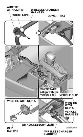
53. Attach one wire tie with clip A to the white tape on the wireless charger harness, secure the wire tie with clip A to the lower tray. If the vehicle has an accessory light, secure the wireless charger harness to the vehicle harness with one wire tie with clip A.
