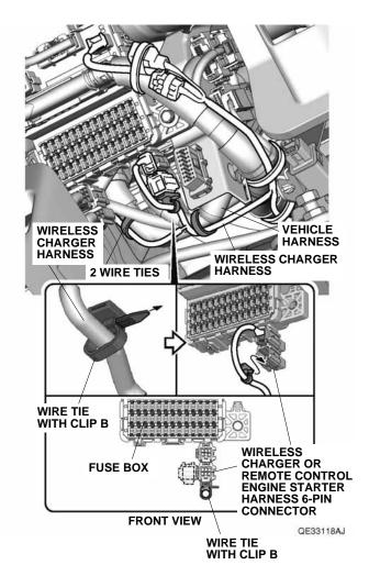
44. Secure the wireless charger harness to the vehicle harness with two wire ties.
