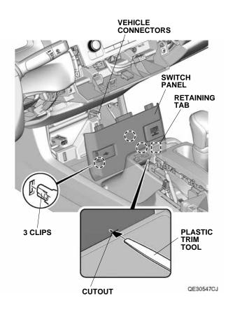
16. If equipped, release the vehicle clip and unplug the vehicle connector.
