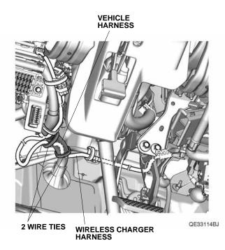
39. Secure the wireless charger harness to the wireless charger harness 6-pin connector with one wire tie with clip B.
