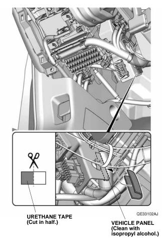
21. Using scissors, cut one urethane tape in half and attach one piece to the vehicle panel.
