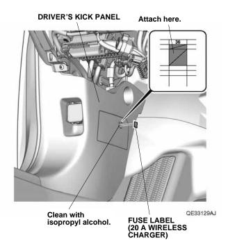
59. Attach the fuse label on the driver's kick panel.
