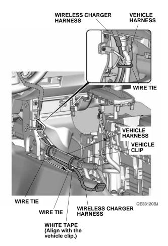
48. Secure the wireless charger harness to the vehicle harness with two wire ties.
