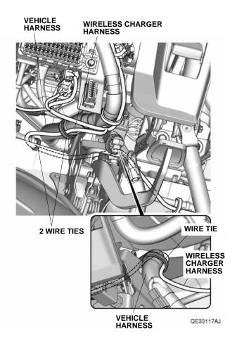
43. Secure the wireless charger harness to the wireless charger harness 6-pin connector with one wire tie with clip B.
